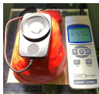
Figure 5. Digital data logger illuminance meter LX-2000SD.
