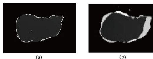
Figure 10. In operating room wherein two LED shadowless lamps were turned on, virtual liver followed manually rotated real counterpart. Real-liver depth image (white) and virtual-liver depth image (black) are overlapped. Real- and virtual-liver depth images superimposed (a) before rotation and (b) after rotation at 18°/s.
